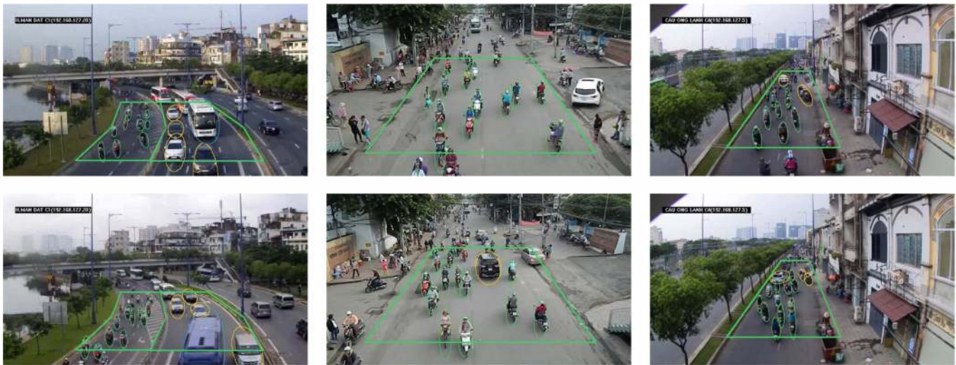
Fig. 6. Examples of occlusion vehicle detection and classification result with three experimental datasets. Green, yellow, blue ellipses respectively indicate light, medium, and heavy vehicles. The 1 st , the 2 nd and the 3 rd column respectively present results from dataset HMD01, NTL01 and COL01.
