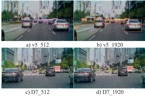
Figure 3: The visualization result of EfficientDet and YOLOv5 in 512 and 1920 resolution input image.
